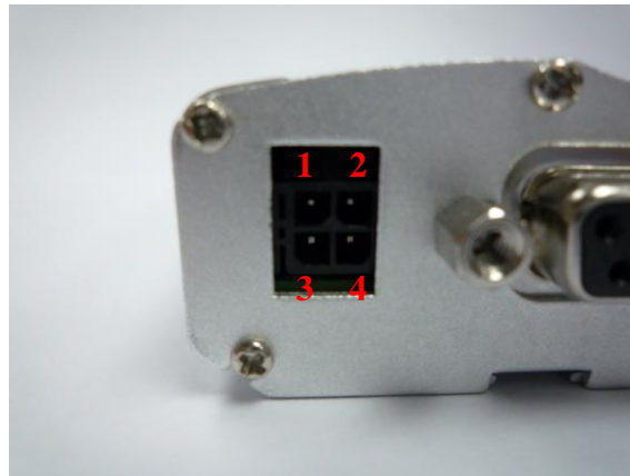
Figure 3: Micro Fit 3.0 Power Supply Socket for TMN-51T
